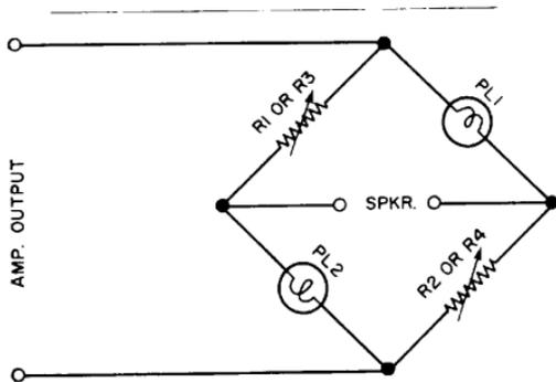
Fig. 1. Basic bridge circuit used.
