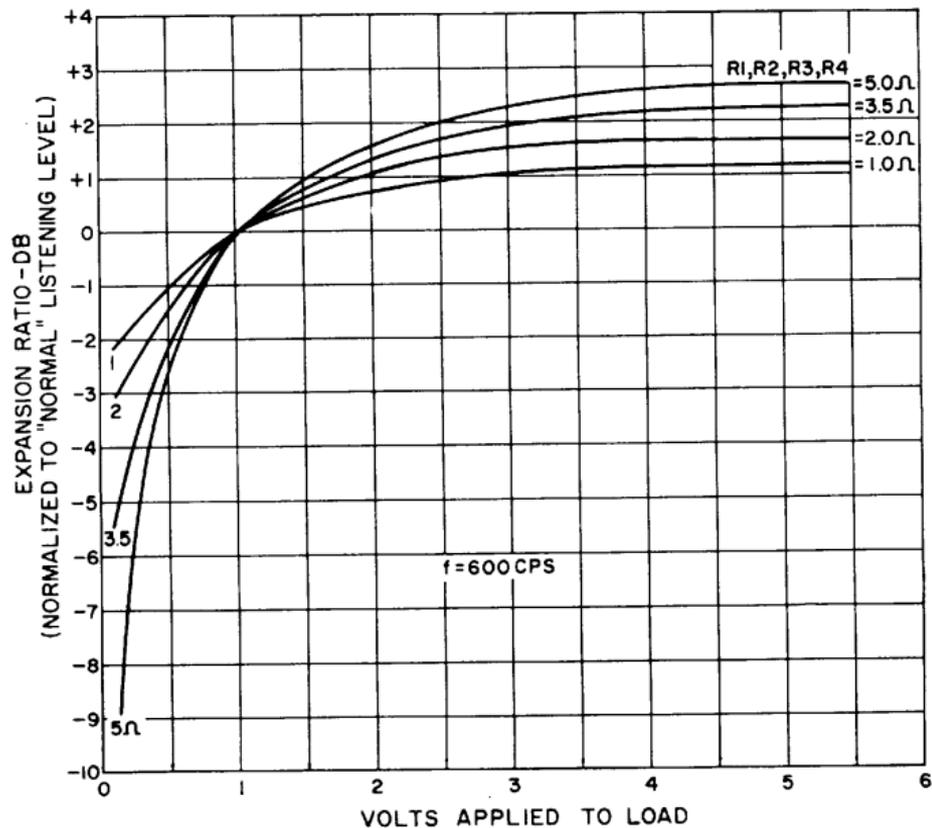
Fig. 4. Range of values of the circuit's input resistance ( $R_X$ ) for various amounts of bridge and lamp resistance when a loud-speaker load with an average impedance of 12 ohms is utilized.
