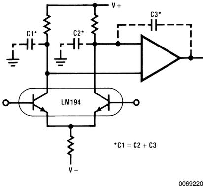
FIGURE 2. High Frequency Power Supply Rejection
