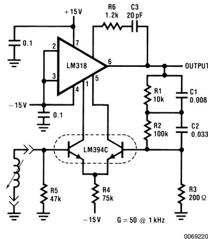
NOTE: Cartridge is assumed to have less than 5 k $\Omega$  DC resistance. Do not capacitor couple the cartridge. R1, R2, and R3 should be low noise metal film resistors.
