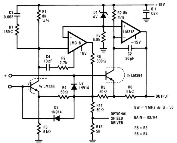
FIGURE 5. Low Drift-Low Noise Instrumentation Amplifier
