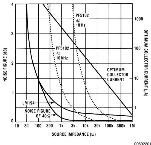
FIGURE 1. Noise Figure vs Source Impedance
