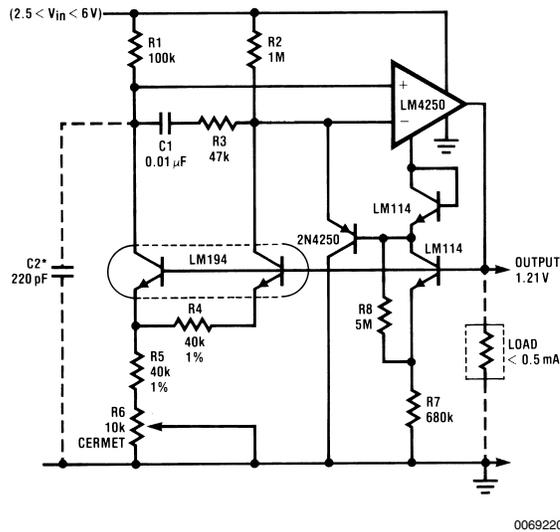
FIGURE 9. Micropower Reference
