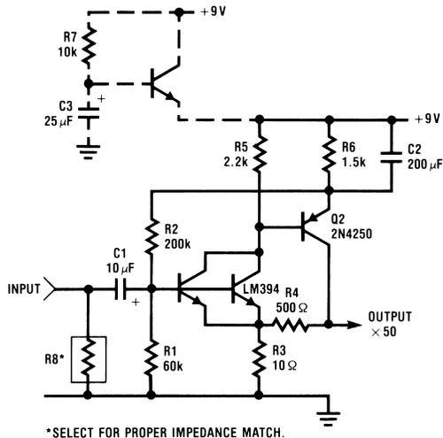
FIGURE 4. Ultra Low Noise Preamplifier
